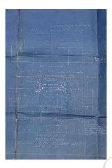
Figure 8.8. This portion of a Carrère and Hastings blueprint shows a profile view of the structure designed to hold the Unknown's remains until the final Tomb could be designed. Note the position of the casket within the base. (National Archives and Records Administration)
